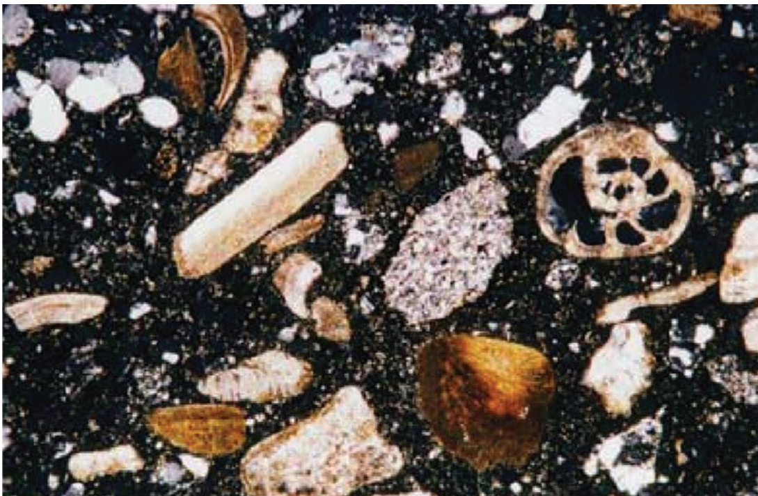
Petrographic image captured of the bridge concrete revealing seashells. Comparable shell material can be identified at the nearby Barleycove beach.
