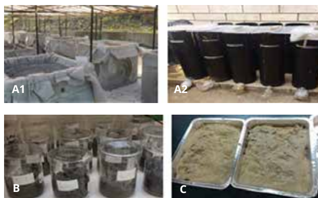
Fig. 3: Examples of mecosocoms (A), microcosms under curing (B) and microcosm after the preparation (before the packaging in the glass backers). [14]
