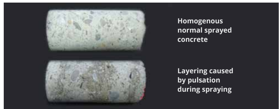
Figure 2: Visible layering in a drilled core, compared to the competent application [4]
