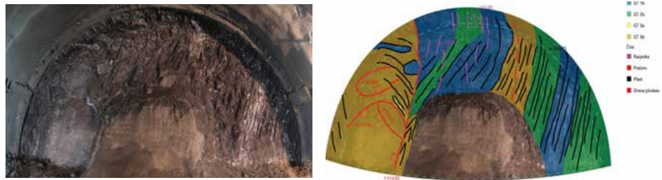
Fig. 8: Popis in fotografija čela kalote na TM 2268,6 (22.11.2022). Description and photograph of the top heading face at TM 2268.6 (22/11/2022)
